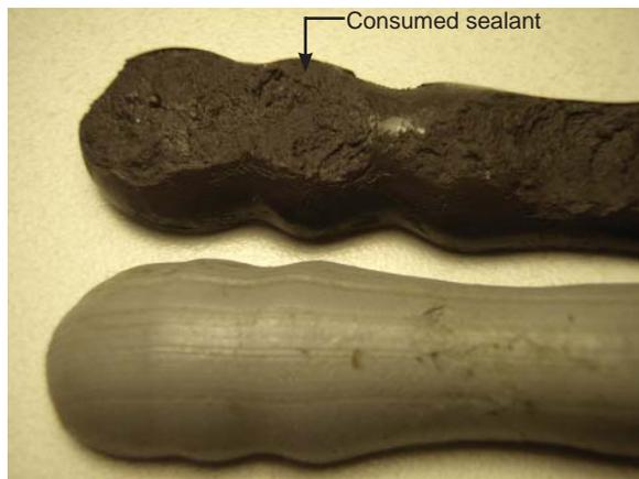
*As a final test, two new silicones were selected based on their chemical composition. Both from the same manufacturer, the upper sealant contains the siloxane compound, while the lower bead contains the titanium catalyst. The snails' preference is clear.*
