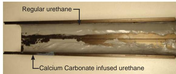
*The second test's results supported the theory that the snails were eating the sealant primarily as a source of calcium. For this test, urethane sealant was chosen specifically for its composition, in that it does not contain calcium. The bead aligned with the blue tape contains the calcium carbonate (white powder), while the other sealant is as sold by the manufacturer.*
